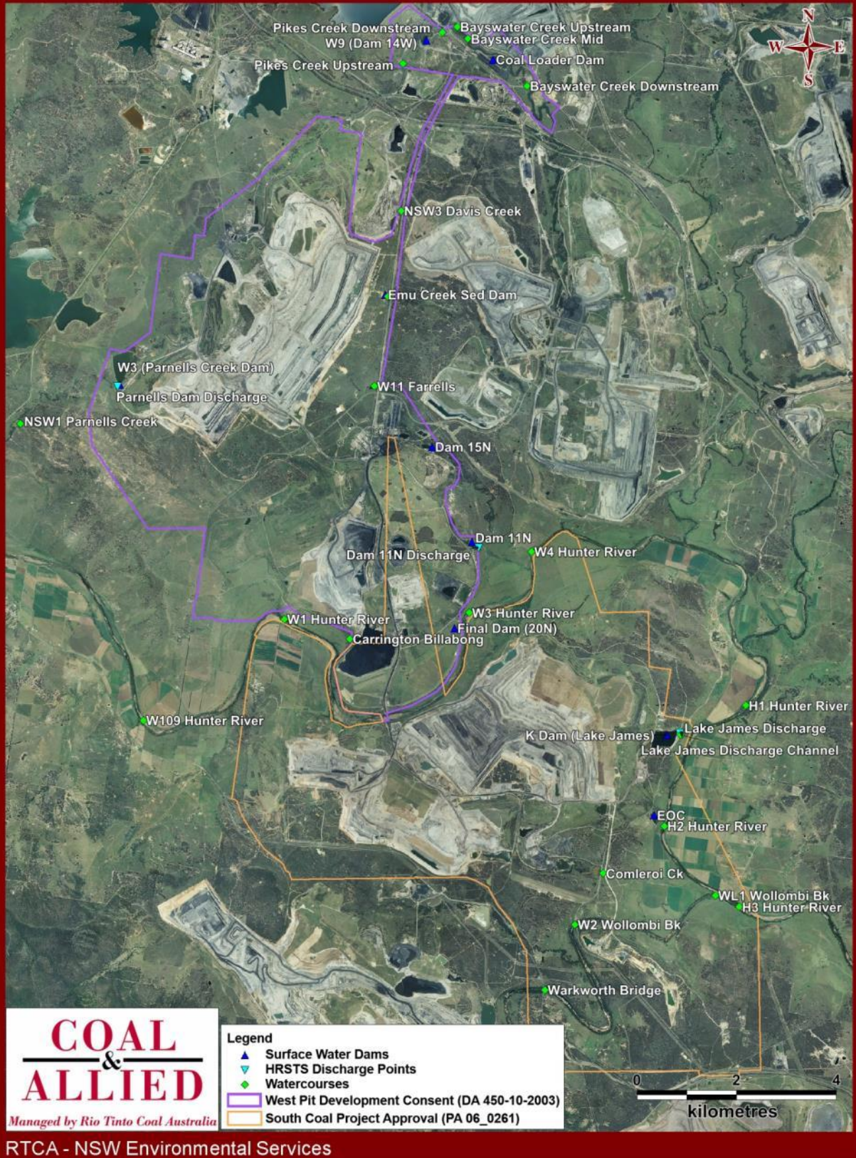
Figure 22: Surface Water Monitoring Location Plan
